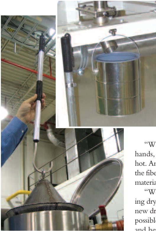
Far left These hooks are designed to easily remove cone-shaped diffuser baskets, which prevent bridging and improve drying efficiencies. Left Stainless steel drop chutes, ergonomically positioned beneath the hoppers, ease contaminant-free materials removal.
