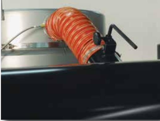
Inlet/outlet Dampers Control Air Flow to each Hopper
