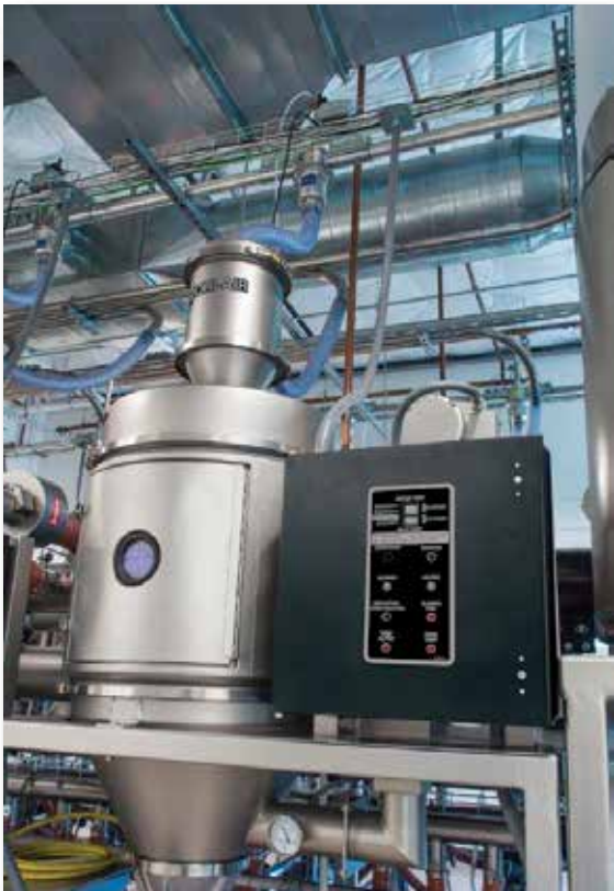
Control locally at CDA2 or from dryer control
