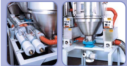
Modular stands bolt together for future expansion
