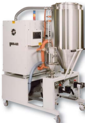
HPD-6 with a 5-lb (2kg) colorant hopper
